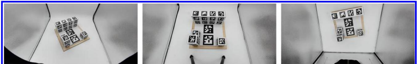
Fig. 5 Example photographs of the ship deck used for feature and 3D point extraction, collected at each of the three camera positions.
