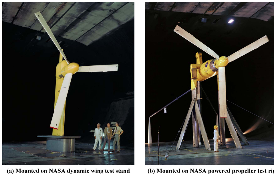
Fig. 2. Boeing M222 tests in NASA Ames 40-ft x 80-ft wind tunnel (1972).
